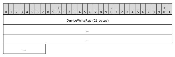
**DeviceWriteRsp (21 bytes):** A DR\_WRITE\_RSP request (as specified in [MS-RDPEFS] section 2.2.1.5.4). The **Length** field of this response is equal to the **Length** field of the Write Request (as specified in [MS-RDPEFS] section 2.2.3.3.4).
