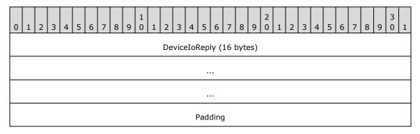
**DeviceIoReply (16 bytes):** A DR\_DEVICE\_IOCOMPLETION header (as specified in <a href="MS-RDPEFS">[MS-RDPEFS]</a> section 2.2.1.5). The **CompletionId** field of this header MUST match the **CompletionId** of a Device I/O Request message that had the **MajorFunction** field set to IRP\_MJ\_CLOSE.
